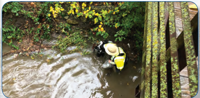
Retrieving a stormwater runoff sample collected using a passive sampler located on the bank of Little Mill Creek in Lenexa, Kansas
