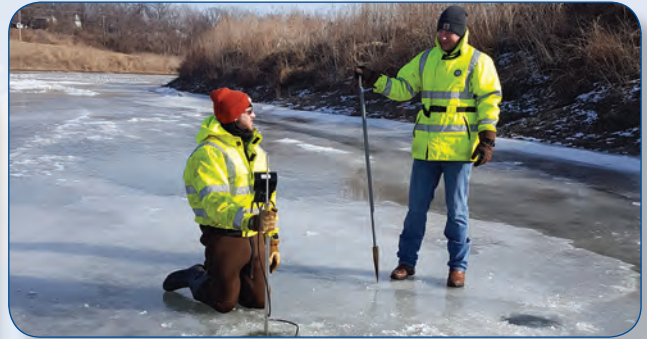
Measuring streamflow under ice conditions using an acoustic Doppler velocimeter
