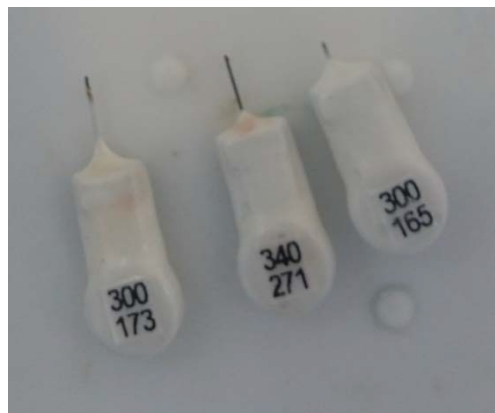
Figure 1-1. Photograph of three Lotek NTQ-2 radio transmitters recovered from tagged fish recollected at the Cowlitz Falls Fish Facility during 2016. The transmitter antenna broke and was lost during the period between when fish were released and when they were recollected.
