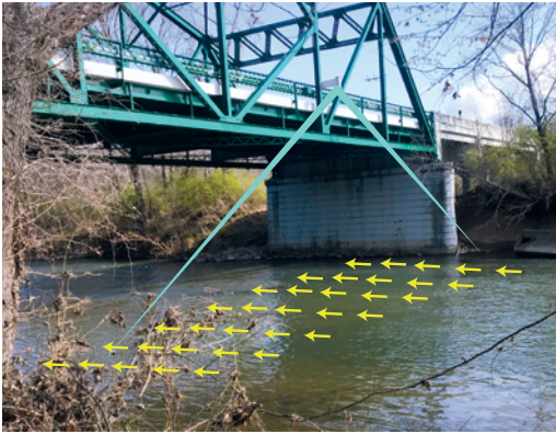
The USGS is advancing the use of large-scale particle-image velocimetry (LSPIV)—a method that uses innovative video analysis techniques—to measure streamflow. Photograph by Mike Woodside, U.S. Geological Survey.
